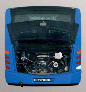
Isuzu Citimark is powered by Isuzu 4HK1 E5S diesel engine, which is qualified for Euro 5 EEV (Enhanced Environment friendly Vehicle) regulation of the European Union. 4HK1E5S is an inline 4 cylinder direct injected diesel engine with a displacement of 5.2 litres. The engine is fitted with a turbo charger and an intercooler in order to boost the engine performance and torque, and it features a cast-iron cylinder block with dry sleeve cylinder liners and a ladder type crankcase.
